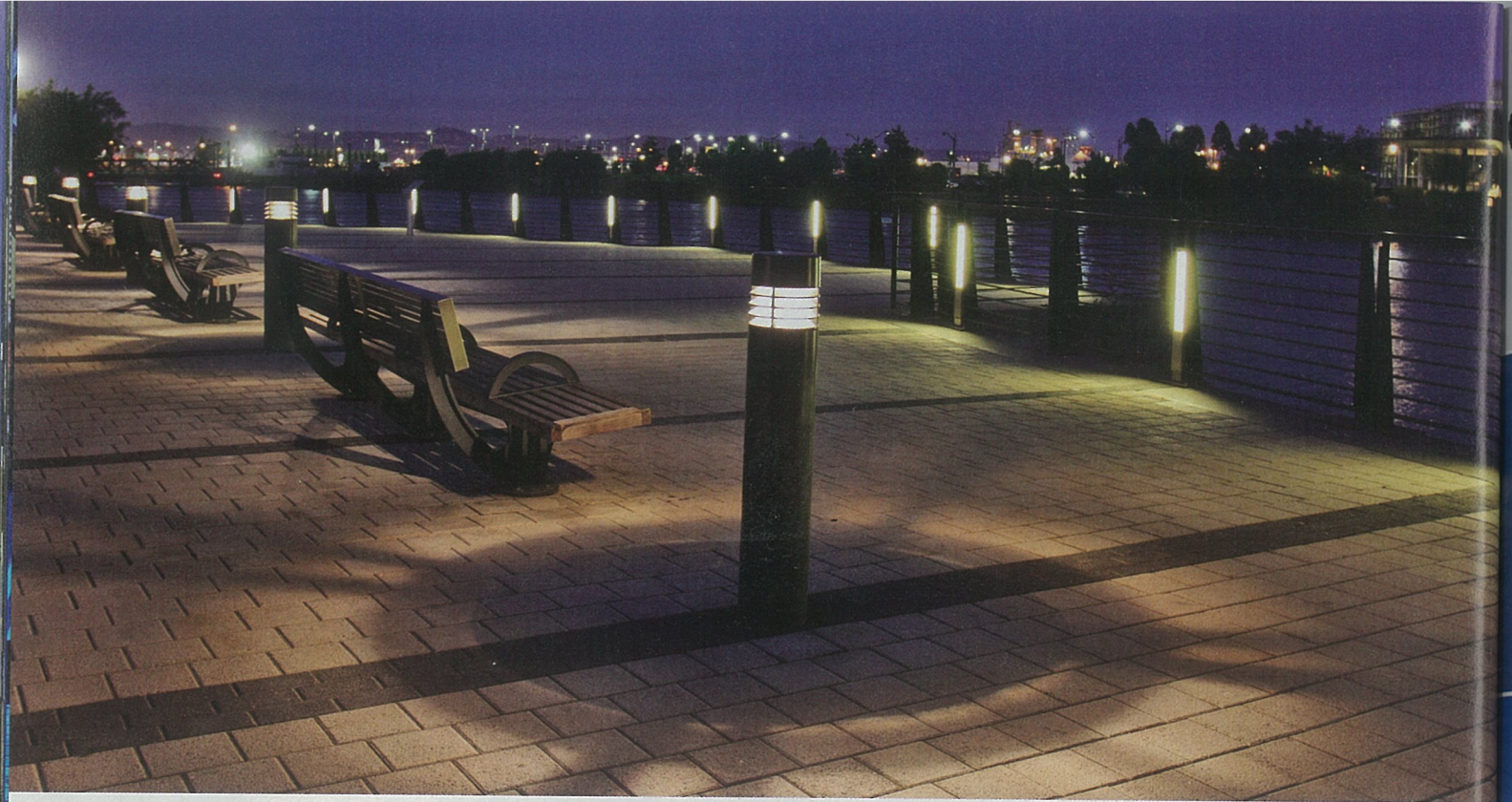
ABOVE: Lighting for the 5th Street Overlook remained low level so as not to obscure the waterfront view of the Mission Bay Development to the south. Custom fluorescent steplight fixtures integrated into the handrail design and louvered bollards provide pools of light that intermingle playfully on the overlook.
