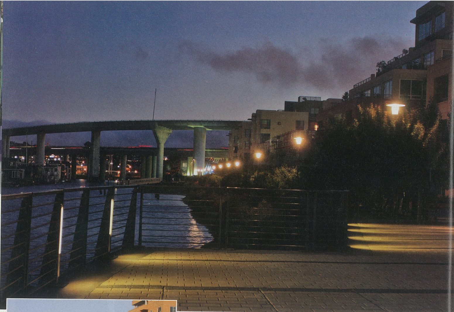
ABOVE: Custom light fixtures, seamlessly integrated into the handrail design, provide low level pools of light onto the esplanade walk. Decorative pedestrian light poles softly illuminate the long walk in between the overlooks.
